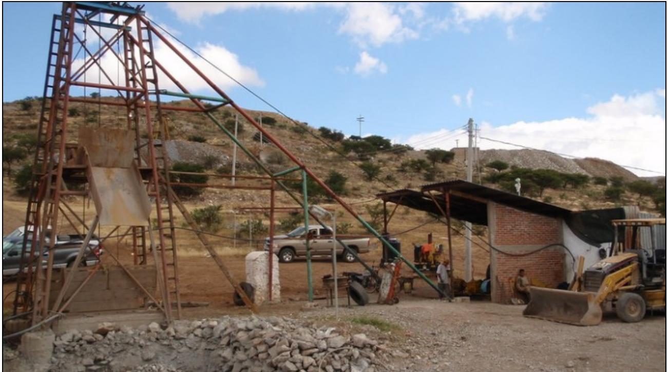
A head frame at Southern Silver Exploration's Cerro Las Minitas project. Credit: Southern Silver Exploration.
